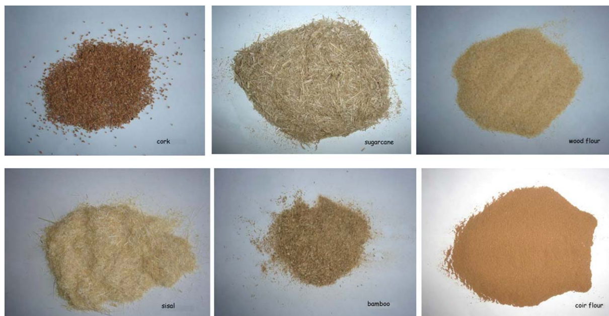
Figure 1 Photographs of the fillers. [Color figure can be viewed in the online issue, which is available at www.interscience.wiley.com .]
